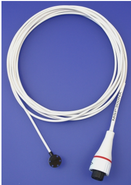
Figure 3: An OxyFlo probe ('MSP300NX' type depicted)
