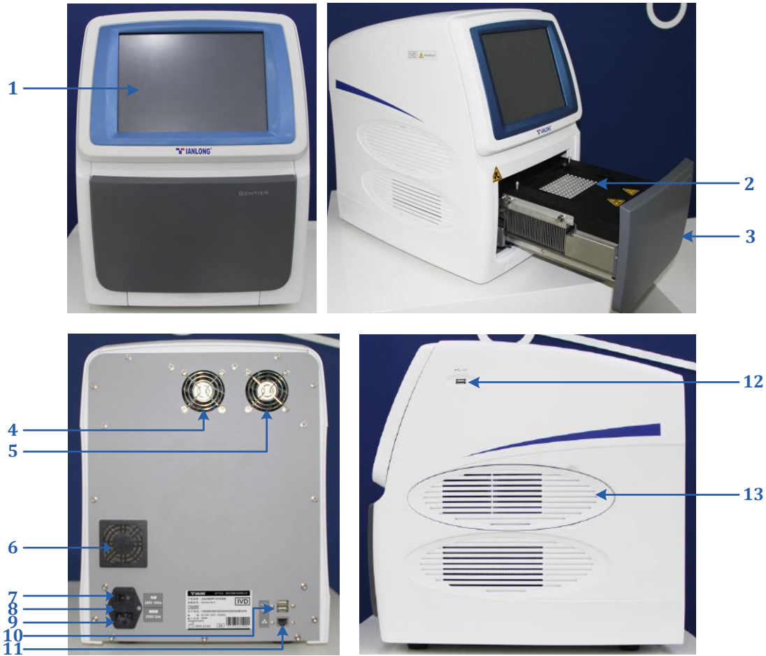
Figure A-1. Gentier Instrument Structure
